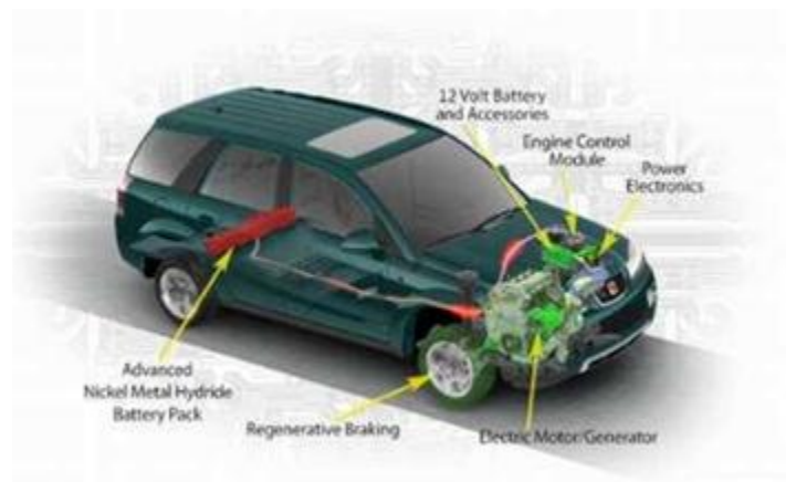
Figure E-2: Saturn Vue Green Line Primary BAS Technology Configuration
