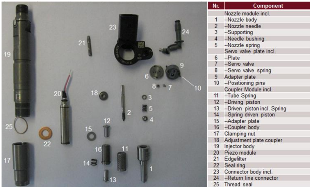
Figure B-3: Initial Level of Injector Teardown
