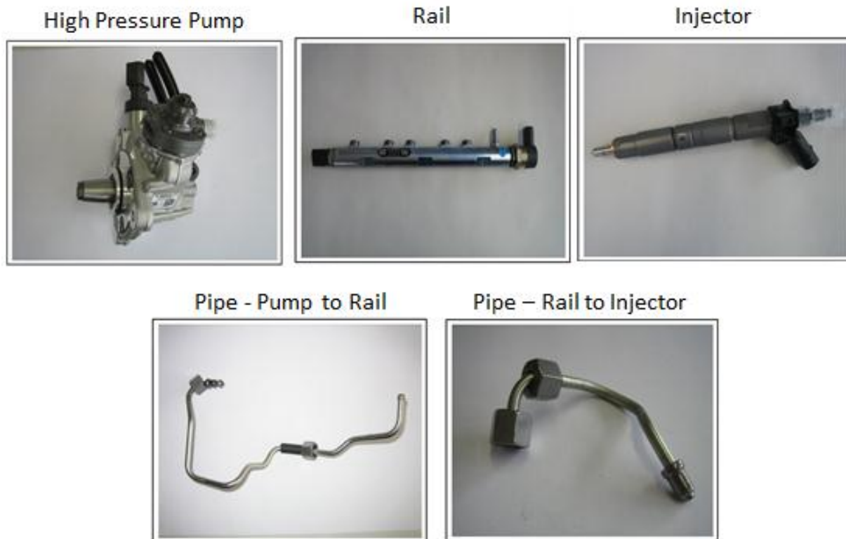
Figure B-2: Sample of Components Removed During High Level Teardown of Fuel Induction System
