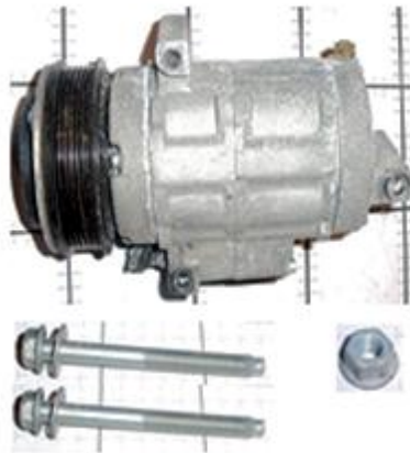
Figure E-5: Belt-Driven Compressor and Mounting Hardware
